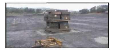
127 SCPT tests were performed on site which confirmed uniformity of the treated PFA at the site. The testing also confirmed an Increase in Cone Resistance to **around 4m bgl.**
